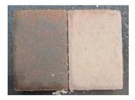
Photo left - ColorScape® EverBold® pavers in left 4 rows. Standard pavers from the same pallet and production run in right hand row. Photo taken several days after manufacture.
