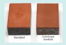
Standard and ColorScape<sup>®</sup> EverBold<sup>®</sup> pavers tested with a concentrated solution of muriatic acid for 2 minutes. Note the etching on the standard paver.
